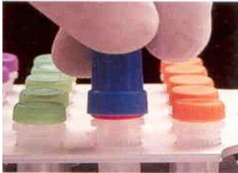
The Micro Tube Tool's larger end is a socket wrench for Screw-Cap Micro Tubes.
