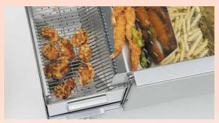
Cooked foods are carried out to the discharge chute in front of the machine. One person can operate.
