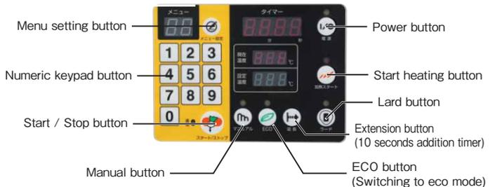
The operation panel at left side has a switch of menu setting, start/stop and extension only.
