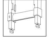
Easy to adjust foot: Handle irregularities on the floor by easily adjusting the foot.
