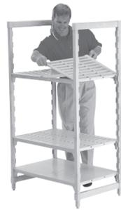
**4** Add an additional unit by connecting two more posts with post connectors and the setting traverses onto the dovetails on the posts. The traverses on the first and second unit share the middle post. Place shelf plates on the traverses to complete the second unit. Add an additional unit in a 90° corner using corner connectors.
