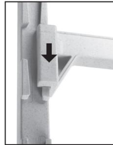
Traverse slides easily down onto dovetails
