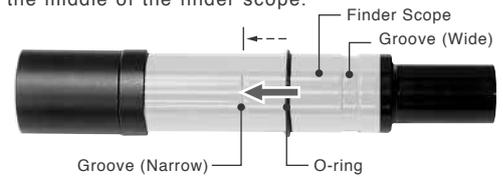
2. Pull up the fixed stud on the bracket ring so that the finder tube can slide into the bracket ring from its eyepiece end. Release the fixed stud into the wide groove on the finder tube.
