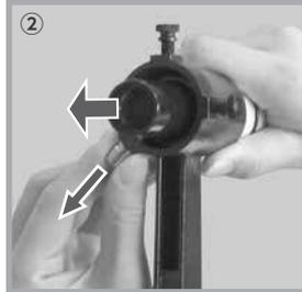
3. Tighten the two adjustment screws so that the finder scope is aligned as shown in the figure.
