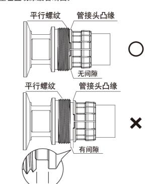
5. Secure the hexagonal part of the nipple with another monkey (motor) wrench and tighten the hexagonal cap nut completely. Tightening the nipple without securing it may cause the nipple to turn at the same time and break the thread for the piping.
